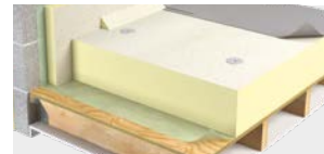
Typical Installation Timber Deck
